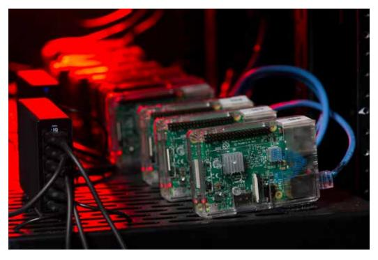
These raspberry pi devices help simulate full-scale grid phenomena using Digital Real-Time Simulators at INL's Energy Systems Laboratory.
