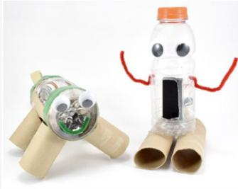
When you turn the battery pack on, it completes an electrical circuit with the motor. This causes electricity to flow in a loop from the batteries through the motor, making the motor spin. Because the motor has a weight attached to its spinning shaft, it wobbles and makes the entire robot's body vibrate, causing it to move. This is the same concept that makes video game controllers and cellphones buzz—they have tiny vibrating motors inside them!
