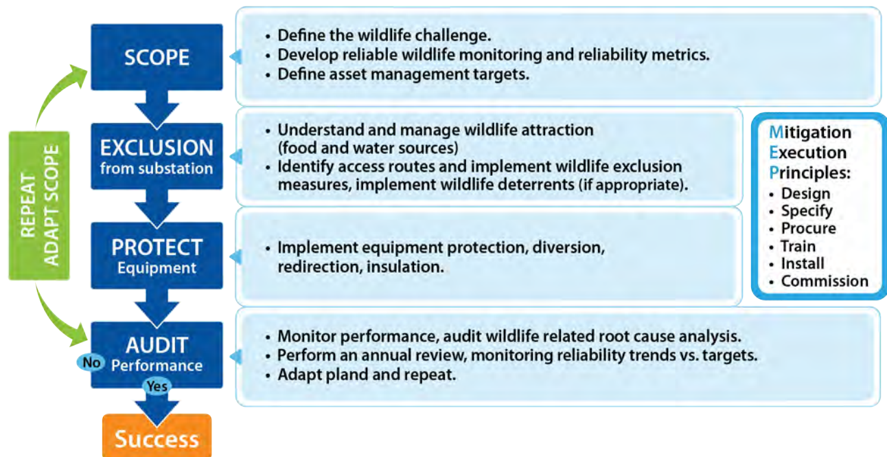
Figure 4. SEPA-R® process for wildlife mitigation at substations.
