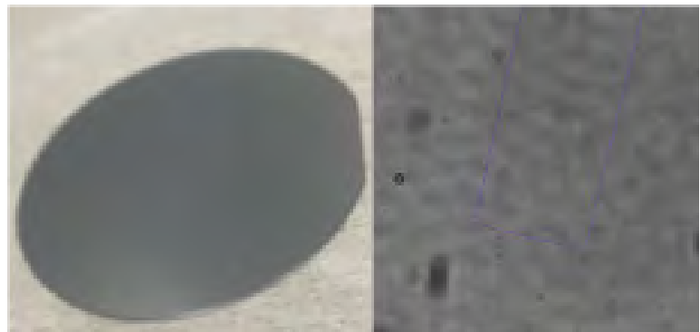
Photos of an entire three inch sample and single feature taken with the custom imaging system where the deposited shadow masked pattern is (a) clearly visible and (b) invisible to the human eye.
