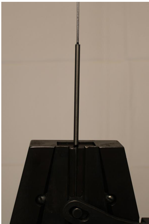
Figure 2: AMC core strand potted in stainless steel tube for testing
