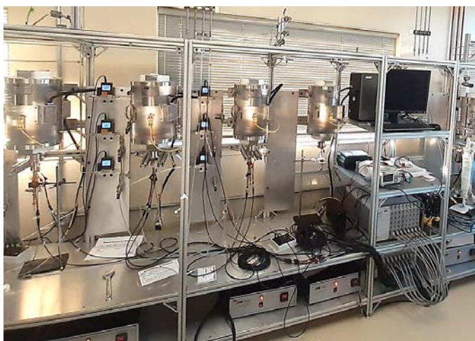
Electrochemistry equipment to develop and test SOEC materials at INL's electrochemical processing laboratory.
