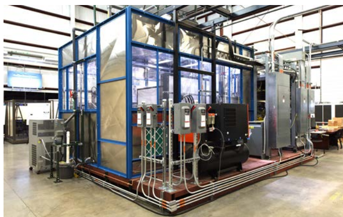
HTE 25 kW stack test station at INL's Energy Systems Laboratory.
