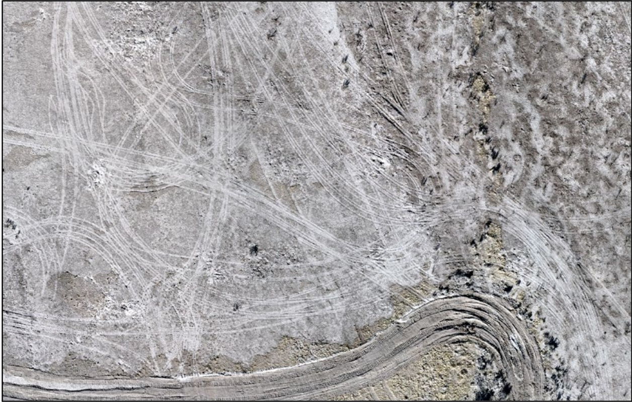
Figure 4-4. Example of two-track density and overlapping routes within a portion of the 2024 Dry Channel Fire on the Idaho National Laboratory Site. A bladed containment line is visible across the bottom of the image.
