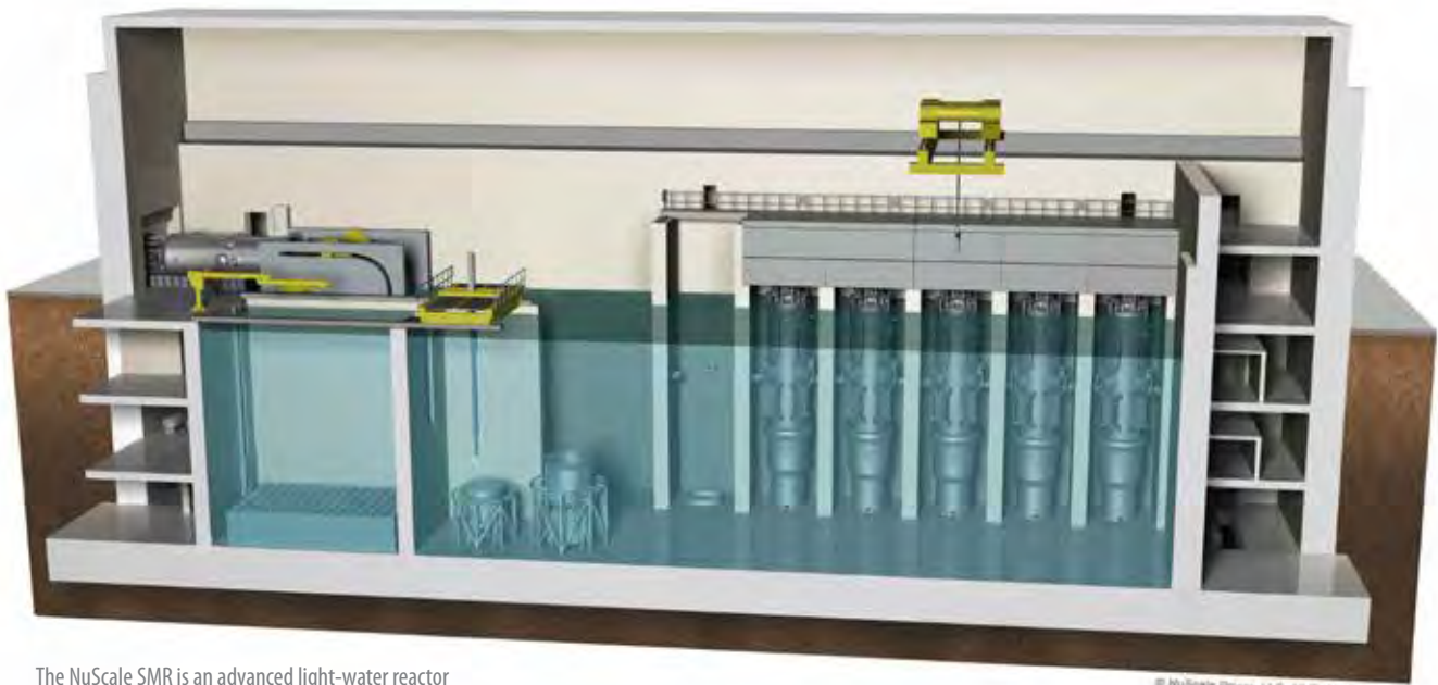
The NuScale SMR is an advanced light-water reactor containing up to 12 modules, each of which is a self-contained unit that operates independently.
