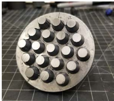
Sample array featuring 19 unique high entropy alloy compositions produced simultaneously using the newly developed parallelized electric field assisted sintering process.
