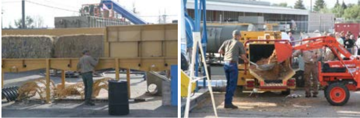
Figure 4. Grinder with one bale of corn stover and one bale of switch grass loaded on the in-feed conveyor (left). Eucalyptus chips are placed on the grinder in-feed conveyor (left).
