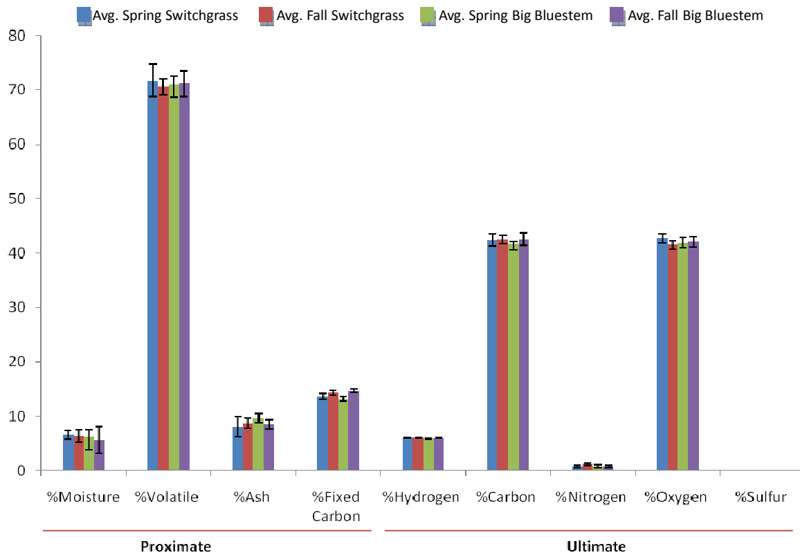
Figure 8. Proximate and Ultimate Analysis results for the 2 grasses from fall and spring harvests. The error bars show the standard deviation of the 4 year harvests. Sulfur content was only 0.07-0.1% in all samples (not visible on the current scale).
