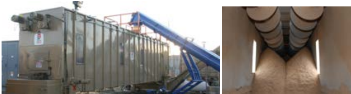
Figure 7. Metering bin showing material inlet on top (left) and inside showing top augers.
