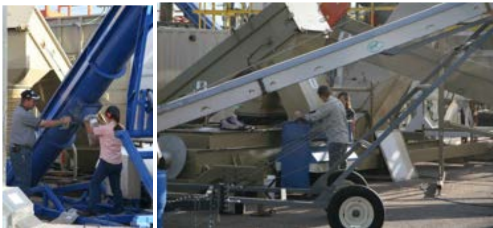
Figure 9. Herbaceous material samples are removed from a conveyor after the initial grinder, then split in a riffle splitter prior to bagging for analyses (left). Other samples of the mixed material are removed from a conveyor just prior to entering the pellet mill (right).
