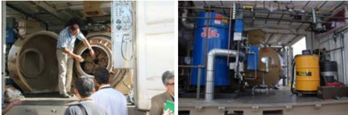
Figure 8. Pellet mill door was opened to show the extrusion process (left). Steam generator is located in an adjacent, connecting cargo container (right).
