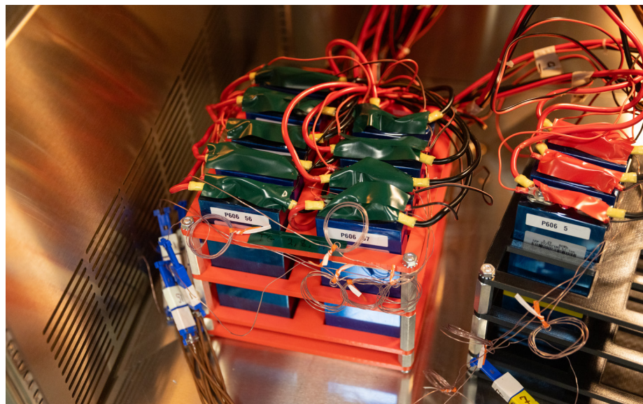
Figure 4: Lithium Iron Phosphate batteries on test at INL in support of the DOE Rapid Operational Validation Initiative (ROVI). This program seeks to obtain predictions for battery health covering 15 years, based on a single year of testing. This is a perfect target for TELEIOS-BATT tools.
