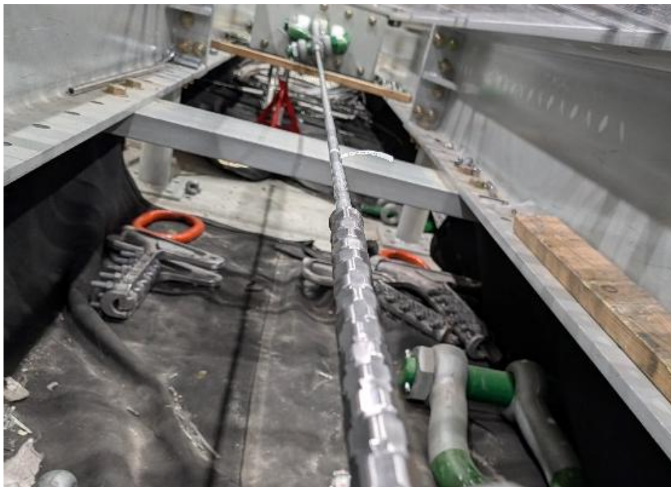
Figure 10. Tensile sample installed in the horizontal tensile test rig
