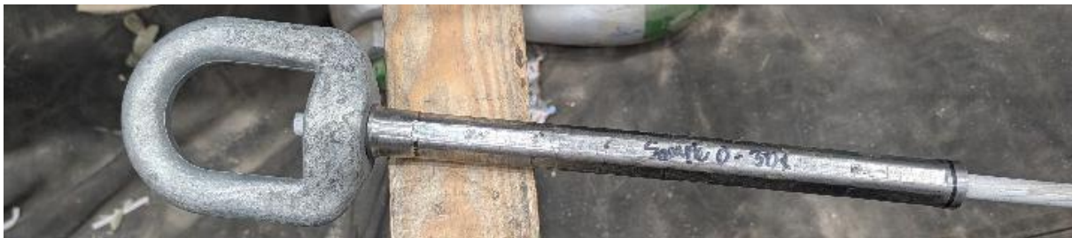
Figure 9. Prepared TS Composite Core with Steel Tube
