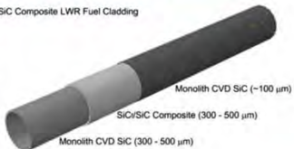
SiC Composite LWR Fuel Cladding
