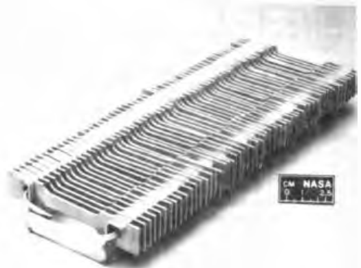
Fig. 1 Typical rack of superalloy tensile-test specimens prior to exposure.
