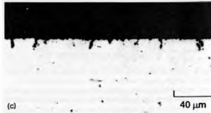
Fig. 9 Effect of long-term 1093 K vacuum exposure on HA 230. Specific weight change as a function of sample position and time (a), near-surface unetched microstructure in the as-received condition (b), and after 10,000 h (c).
