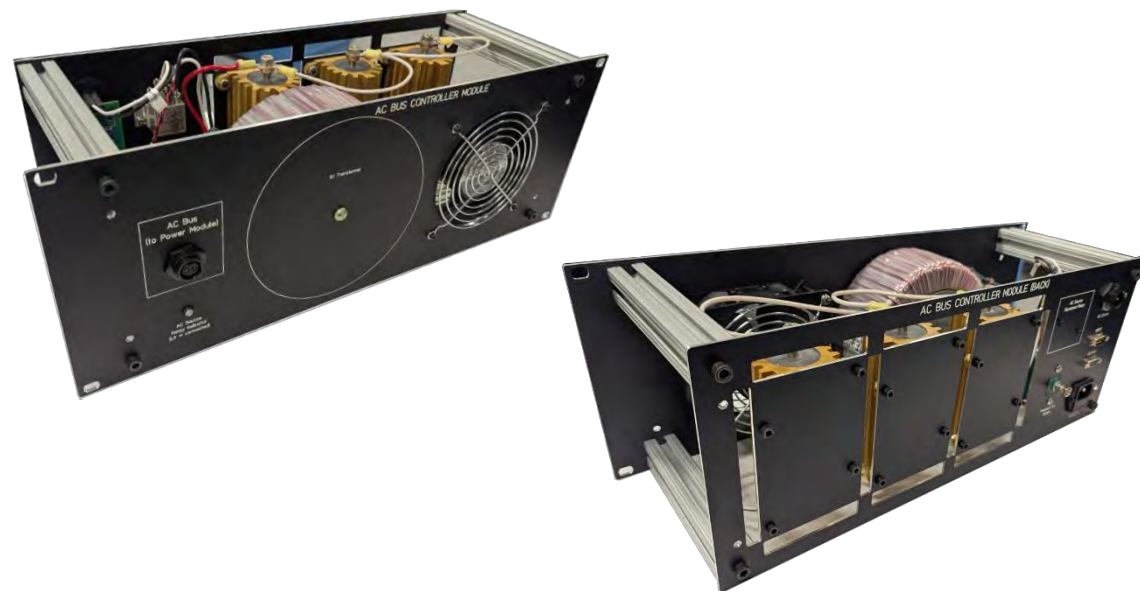
AC Bus/load module front and rear
