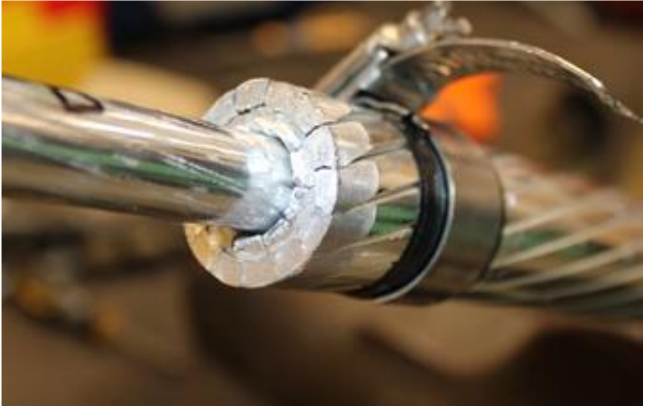
Figure 13: Photo of the Core of Sample 2 prior to Dead-end Installation
