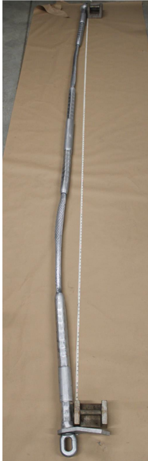
Figure 2: Initial Condition of Sample 3 – Crimped without Rotation
