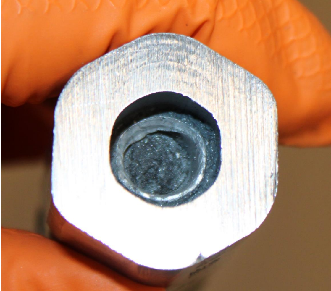
Figure 15: Sample 2 - Location of Failure - Inside of Steel Pin (1 of 2)
