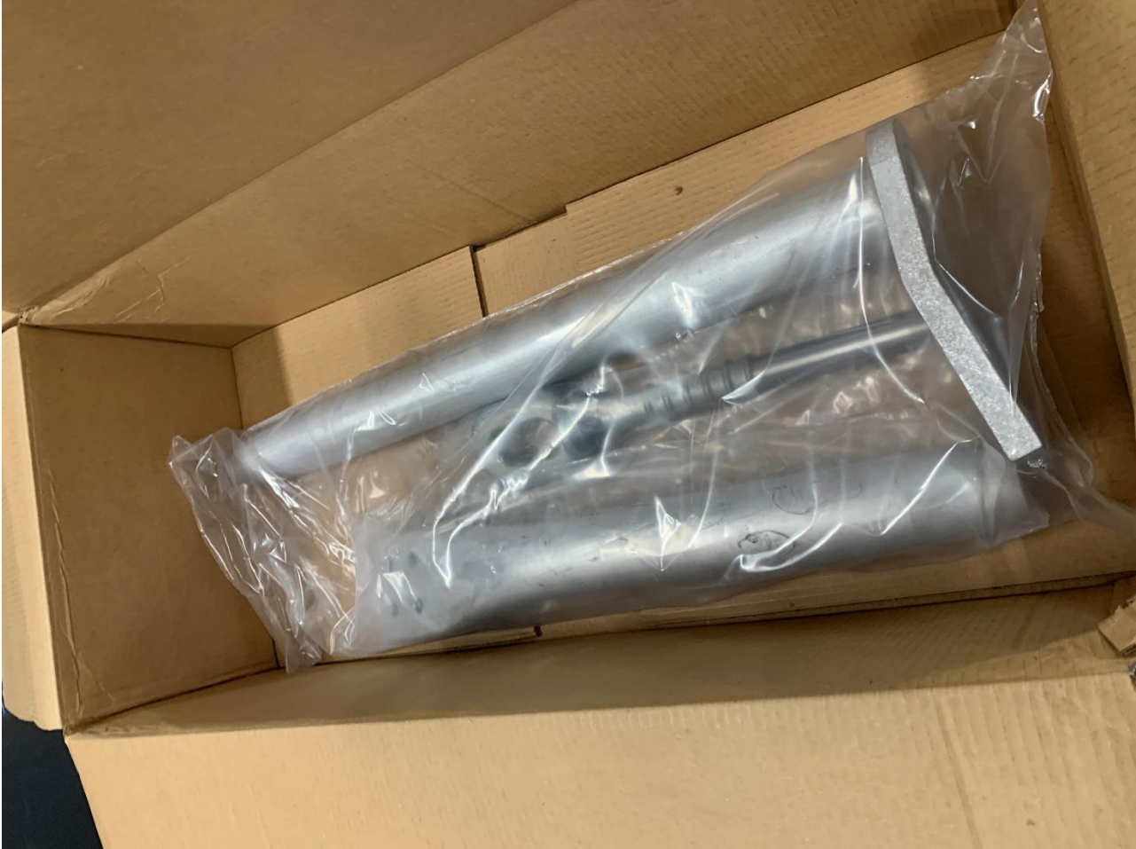
Figure 3: Typical as Received Condition of AFL Deadends, B135010-Y-TS
