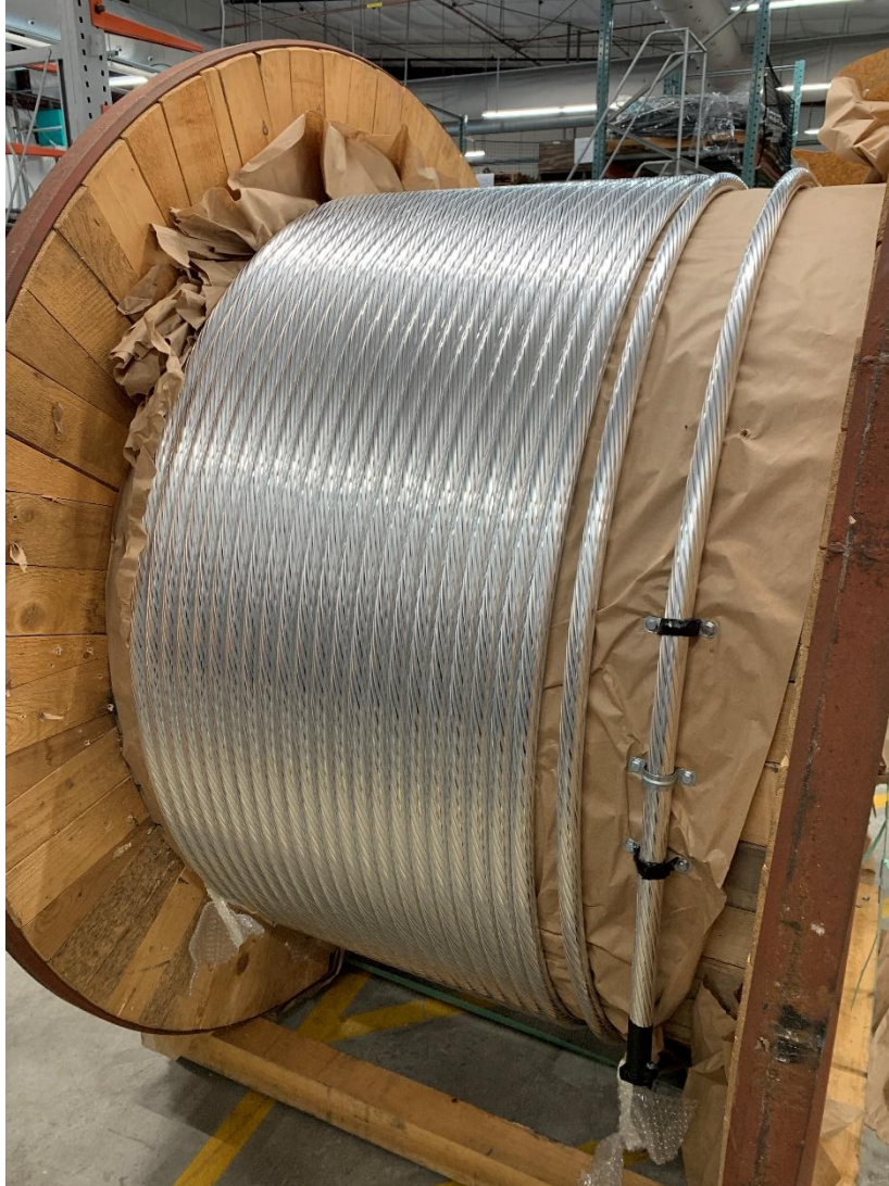
Figure 4: As Received Condition of TS Conductor
