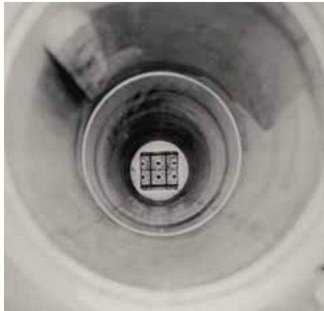
The view toward the core of the MTR through a beam hole.
