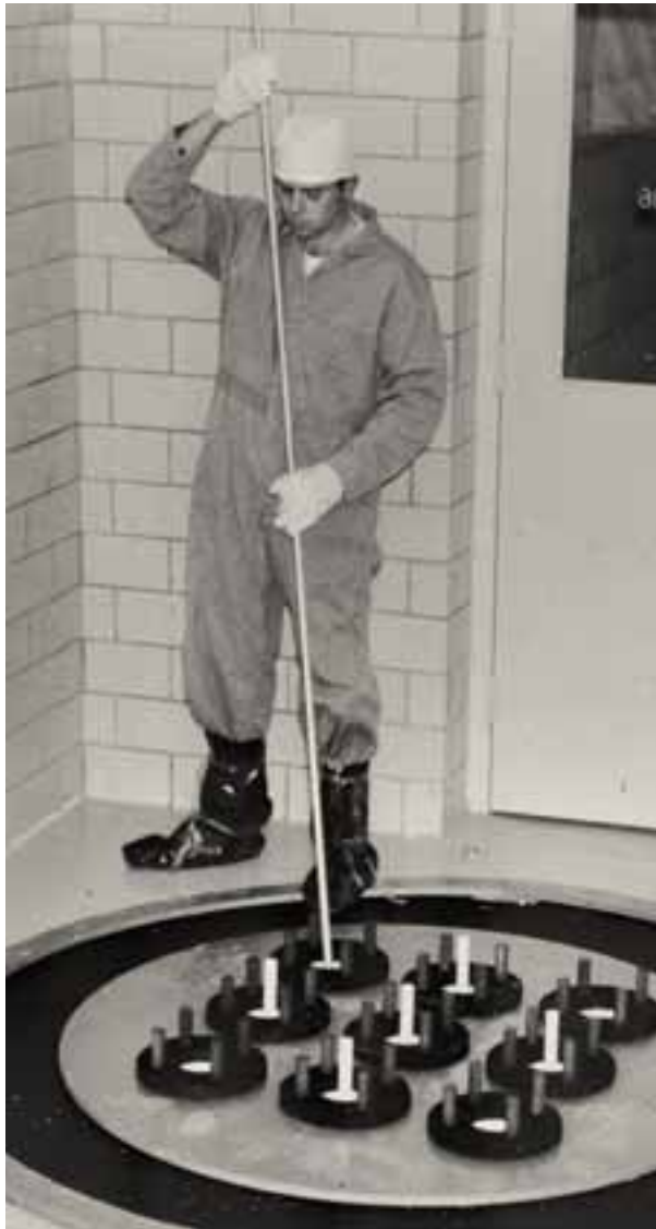
A mockup of the SL-1 reactor top. Analysts tried to determine where the three cadremen were standing at the moment of the accident.
