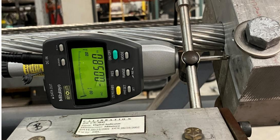
Figure 2: Dial Indicator at Floating End of Gage Rod
