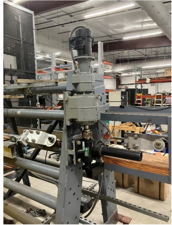
Figure 1: Buffer Springs and Load Cell (Left), Motor-Driven Actuator (Right)
