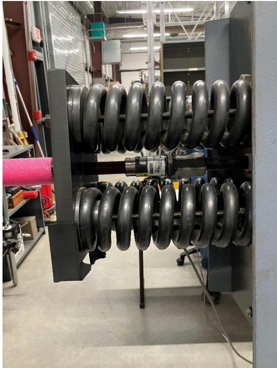
Figure 1: Buffer Springs and Load Cell (Left), Motor-Driven Actuator (Right)
