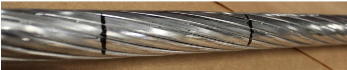
Figure 7: Imprints from the 150 lb/in Crush Load
