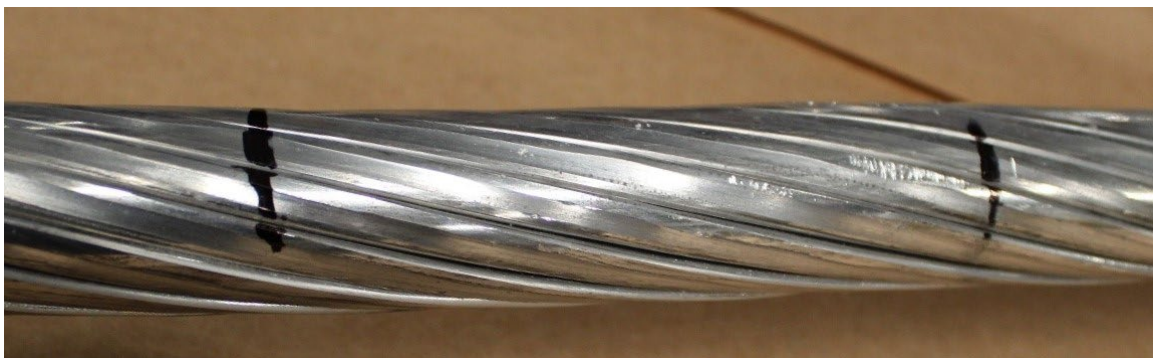
Figure 5: Abrasions from the 100 lb/in Crush Load
