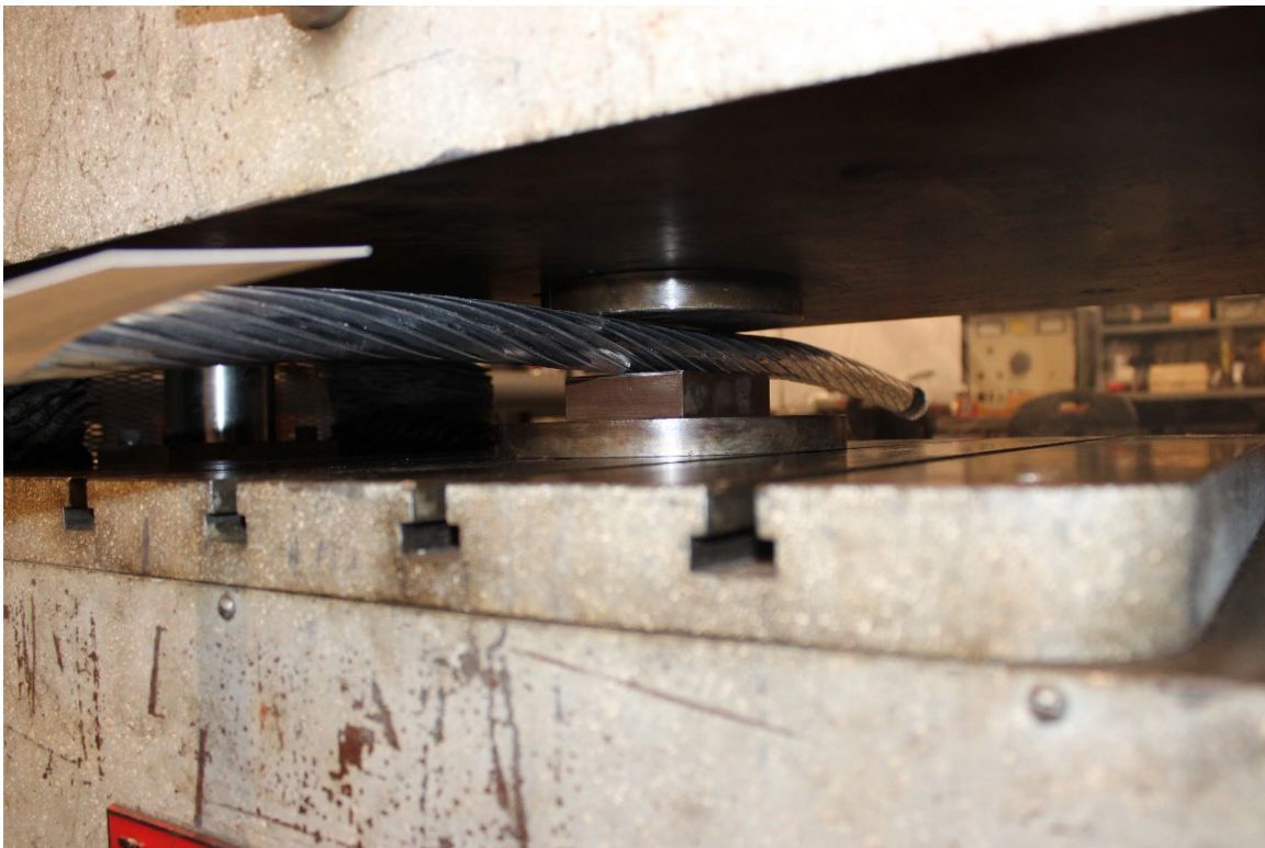
Figure 1: Conductor Crush Test Apparatus
