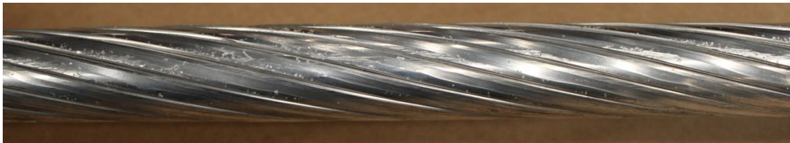
Figure 4: Abrasions from the 75 lb/in Crush Load
