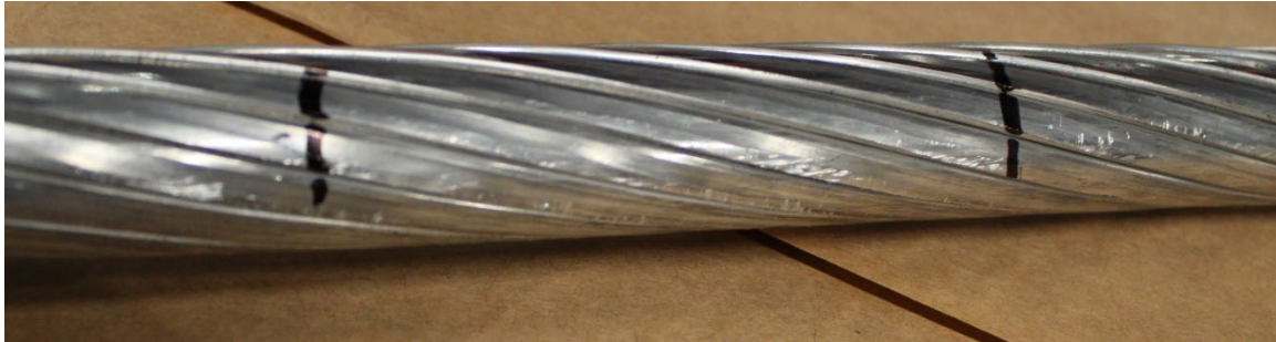
Figure 6: Abrasions from the 125 lb/in Crush Load
