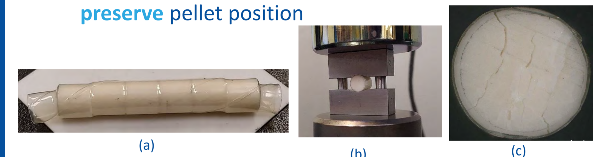
Figure 7: Photo of (a) pellets with mylar wrapping, (b) mechanical compression of individual pellet, and (c) resulting separation-crack formation
