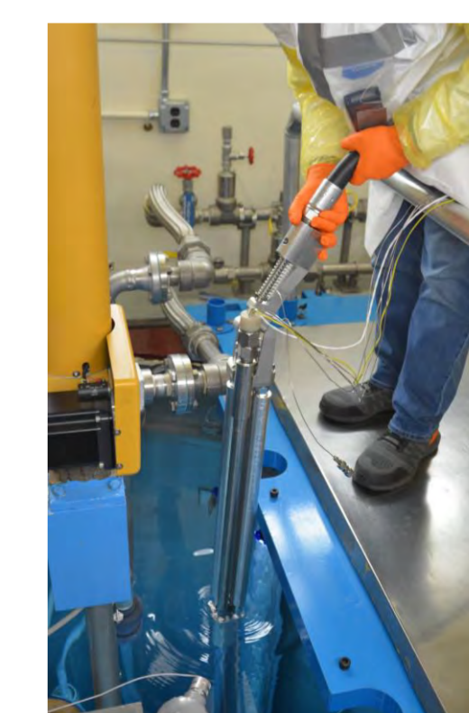
← Inserting the experiment in the reactor
