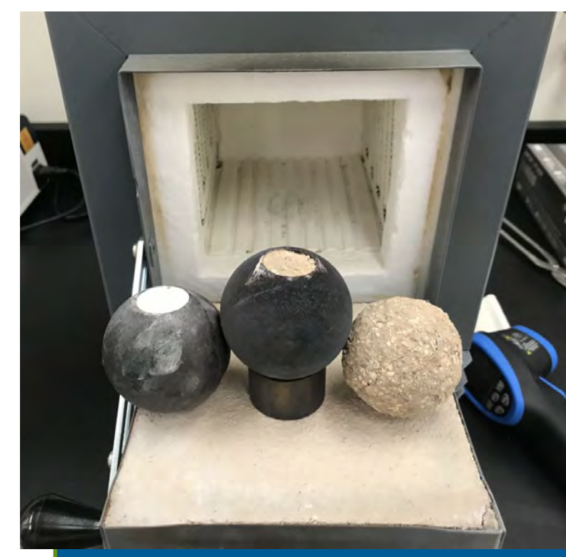
From left – right, Thermogenic Cement spheres, before heating (silver), after heating (dark grey), and the core material without metal casing.
