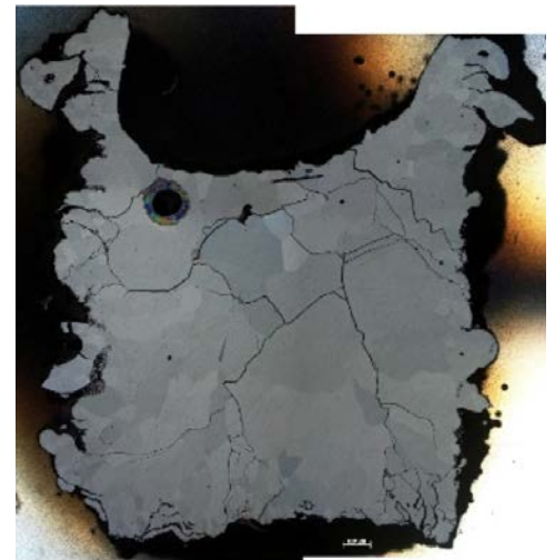
Optical image on longitudinally sectioned fabricated depleted \text{UO}_2 fuel pellet via a directed energy-deposition technique. This image shows intergranular and transgranular cracking due to the presence of high residual stress.
