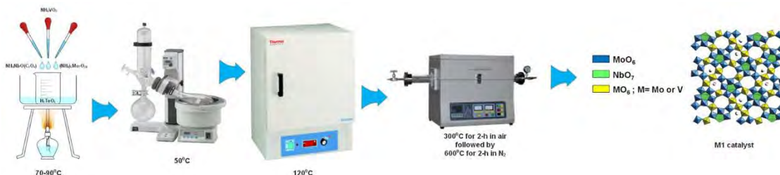
Figure 1. M1 catalyst synthesis by dry-up method.
