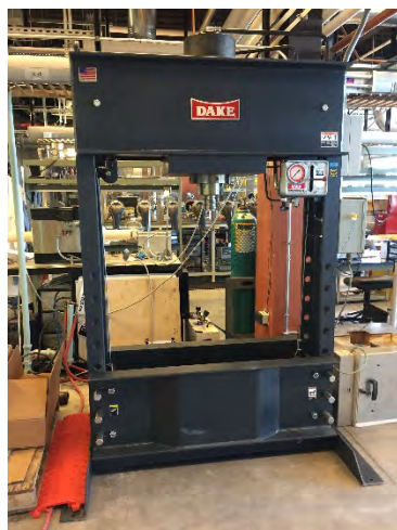
Figure 3. Hydraulic press that is used for loading in the ECAP experiment setup. The maximum load is 150 tons.
