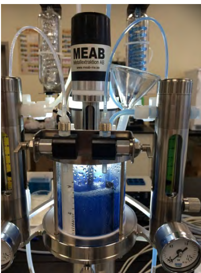
Figure 1. Lamp oil/acidic water experiment in AKUFVE.
