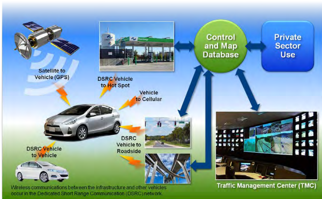
Figure 1. Overview of vehicle-to-vehicle and vehicle-to-infrastructure.
