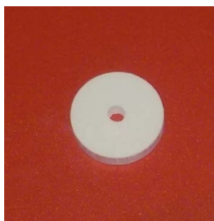
Figure 4. Air-sintered oxide precursor prior to its electrochemical reduction (oxide powder size = <325 mesh, sintering temperature = 975^\circ\text{C} , and duration = 5 hours).
