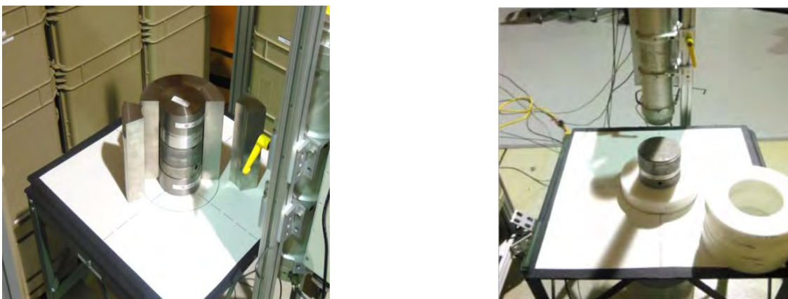
Figure 1. Test setup for interrogating highly enriched uranium (HEU) assemblies. The photograph on the left shows two HEU disks in contact with each other within a 5-cm thick tungsten shell (some parts removed to see the inside). The photograph on the right shows the same two HEU disks, this time with a 2-cm thick aluminum disk in between them; 5-cm thick polyethylene rings are placed to the side prior to being lowered around the HEU.
