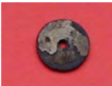
Figure 5. State of the reduced pellet, partial silvery white color on the surface of the reduced pellet was solidified calcium chloride (electrolysis temperature = 900°C, electrolysis duration = 31 hours).
