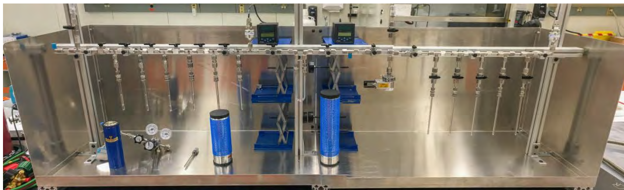
Figure 1. INL's ^{14}\text{C} sample preparation manifold system constructed under this project.
