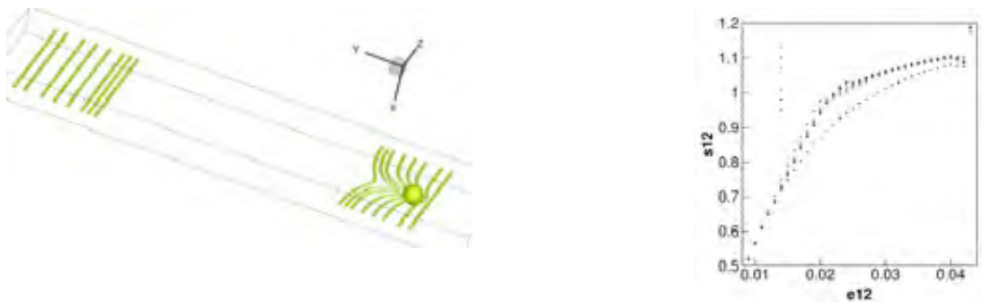
Figure 4. Phase-field simulation of interaction of an edge dislocation with a copper precipitate in iron (left) and resulting increase in the flow stress (hardening) (right).
