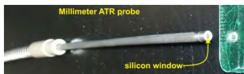
Figure 2. Photograph of the miniature attenuated total reflectance infrared probe.
