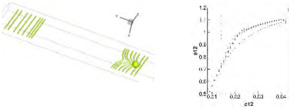
Figure 3. Phase-field simulation of interaction of an edge dislocation with a Cu precipitate in Fe and the resulting increase in the flow stress (hardening).
