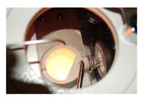
Figure 1. Vacuum-induction melting buttonsized alloy compositions for rapid evaluation of properties.
