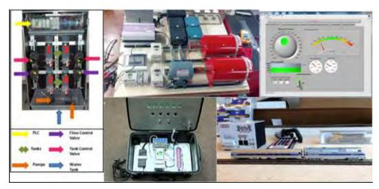
Figure 1. A collage of the enhancements to the testbed for machine learning security experiments include: (clockwise from top left) four tank control, Grid in a Box prototype, control screen for Grid in a Box, the scale model layout of train, and the environmental control system.
