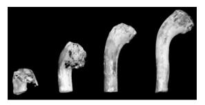
Figure 1. Residual projectiles that were captured after perforating targets were analyzed using the Residual Mass method.
