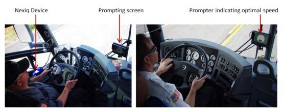
Figure 6. Prompting system installation on an INL Integrated Transportation Services D-series motorcoach (September 2013).
