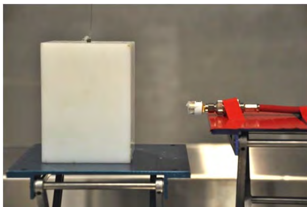
FIGURE 1. The configuration of the ^{252}\text{Cf} source and CVD-diamond detector. The left photograph shows the slightly moderated ^{252}\text{Cf} source and the CVD-diamond detector. The right photograph shows the bare ^{252}\text{Cf} source and the CVD-diamond detector.
