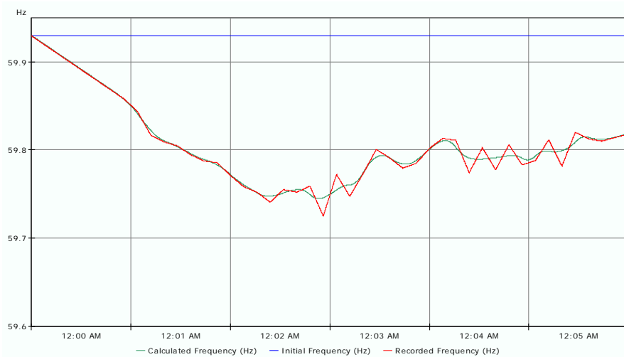
FIGURE 1. Frequency as a function of time for the simplified MEGS model compared to actual data.
