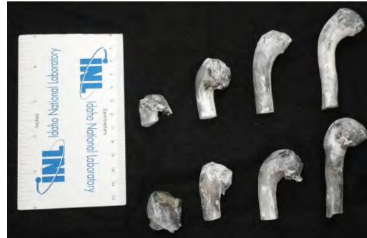
FIGURE 1. Residual projectiles that were captured after perforating targets.
