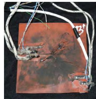
FIGURE 2. A polymer layer with embedded thermocouples to measure temperature during ballistic impact.
