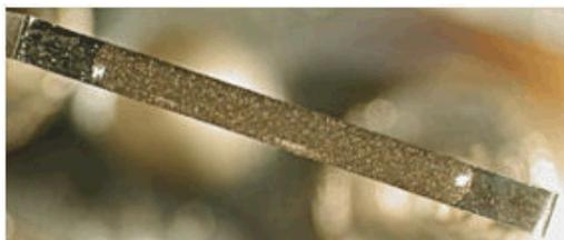
FIGURE 3.  $\text{LaB}_6$ /PIE mixture affixed to a filament.
