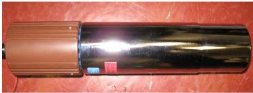
FIGURE 3. Developed special integrated NaI (Tl) detector for DUO<sub>2</sub>.
