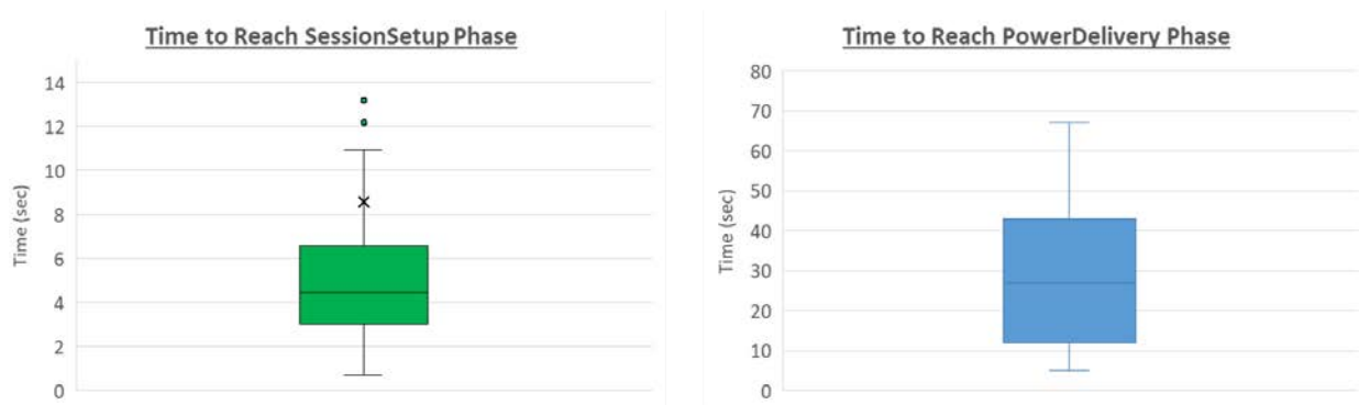
Figure 3. Times to reach Session Setup and Power Delivery phases
