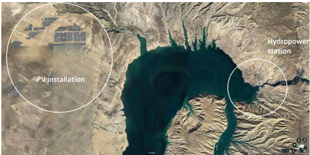
FIGURE 2.25. Satellite image of Longyangxia hybrid hydro/PV power plant
