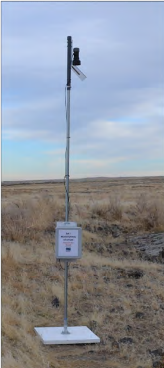
Figure 9-13. Typical Passive-acoustical Monitoring Station for Bats with a Microphone Mounted at the Top. (These devices record the echolocation calls of bats and were installed at cave openings and facility wastewater ponds.)
