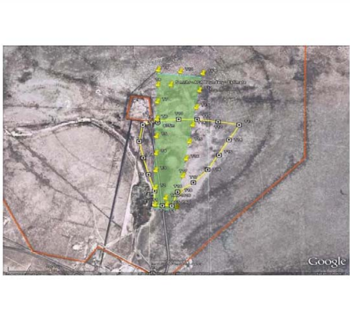
Figure A-8. Example of possible layout for the Intrusion Detection System around the very high radiation area. Examples for the location of the IDS perimeter at the 5 mrem/hr boundary for an INL accelerator. This IDS system has small tower that can be located about 700 feet apart. These towers are small and self contained; receiving power via photocell mounted on top of the tower and transmits its status wirelessly. These towers are about 6 feet tall, and have a very small footprint. Two
