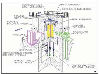
Figure 2. Schematic diagram of a transient test reactor with an experiment inserted into the center of the reactor core.
