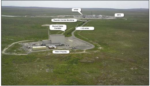
Figure 4. TREAT Facility (foreground) with Reactor Control Building, MFC and HFEF (background). The TREAT Facility and the Reactor Control Building are part of MFC.
