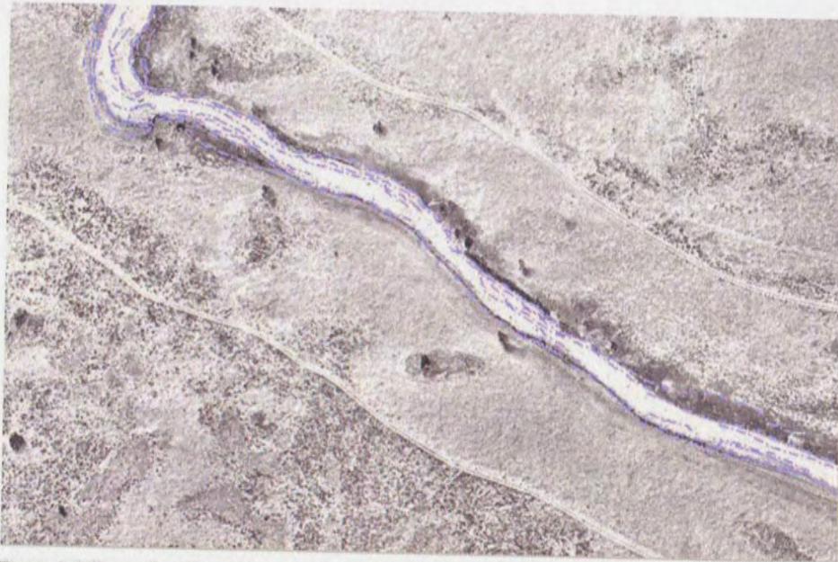
Figure 2-6 Example of breaklines used to aid in definition of Big Lost River channel in 2000 project photography. Dot-dashed lines are breaklines added in stereo models to improve definition of channel features and banks. Smooth-textured areas adjacent to river channel were burned. Area in lower left part of figure with variable texture was unburned; similar areas in upper right were partially burned. Channel reach located in NE1/4, Section 6, T2N, R29E, about 2 miles downstream of the INEEL Diversion Dam.
