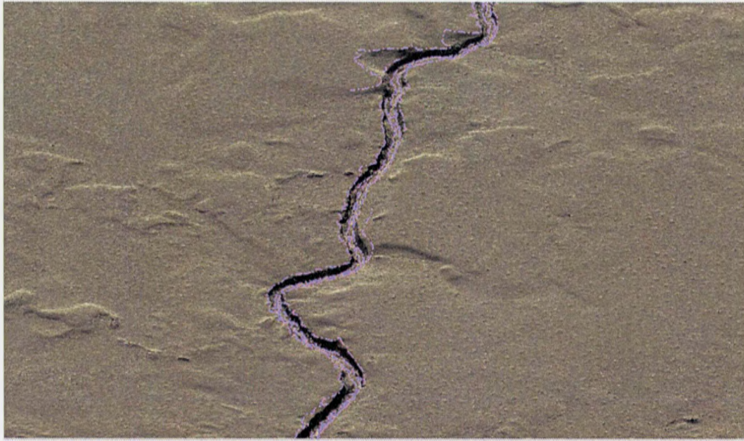
Figure 4-7 Oblique view of breaklines on rendered image of segment of Box Canyon.
