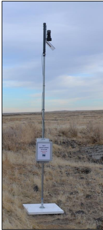
Figure 2. A passive-acoustical monitoring station for bats (about 10 ft.) with a microphone mounted at the top. A gray box (11 x 13 x 6 inches) is mounted to the pole about 3 ft. from the base (2 x 2 ft.). The gray box has a sign attached to it stating that the device is a bat-monitoring station and providing contact information. These devices record the calls of bats.
