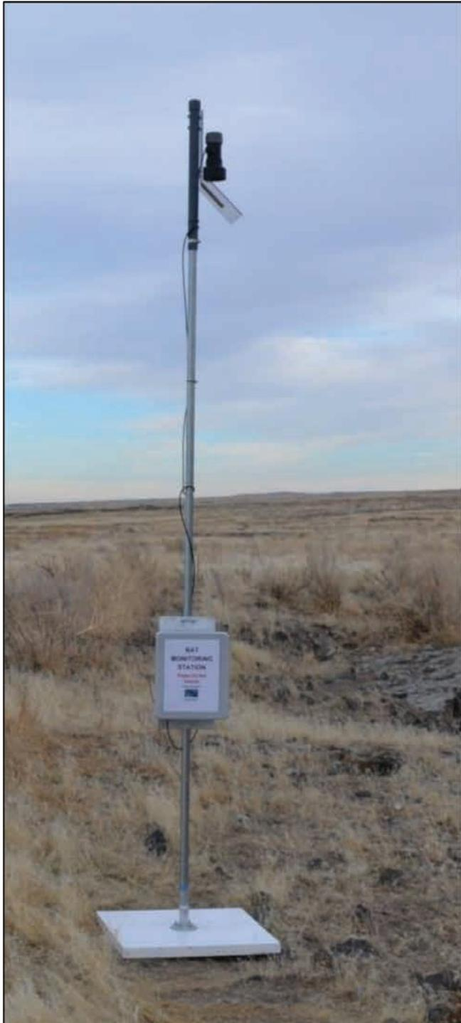
**Figure 8-12. Typical Passive-acoustical Monitoring Station for Bats with a Microphone Mounted at the Top.** (These devices record the echolocation calls of bats and were installed at cave openings and facility wastewater ponds.)
