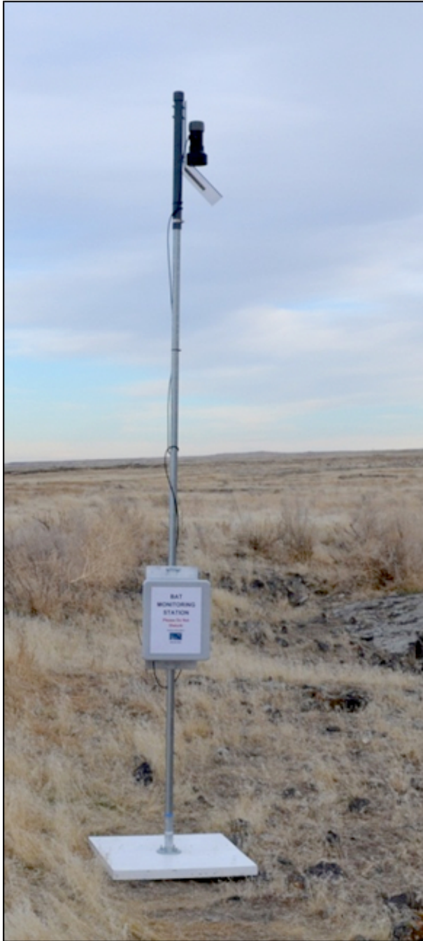
Figure 9-12. Typical Passive-acoustical Monitoring Station for Bats with a Microphone Mounted at the Top. (These devices record the echolocation calls of bats and were installed at cave openings and facility waste-water ponds.)
