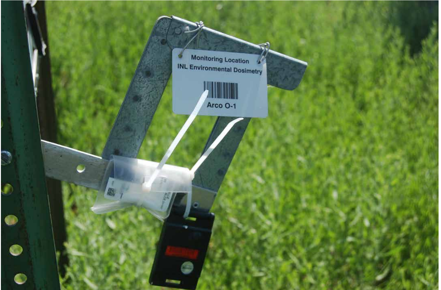
An optically stimulated luminescent dosimeter (OSLD).
