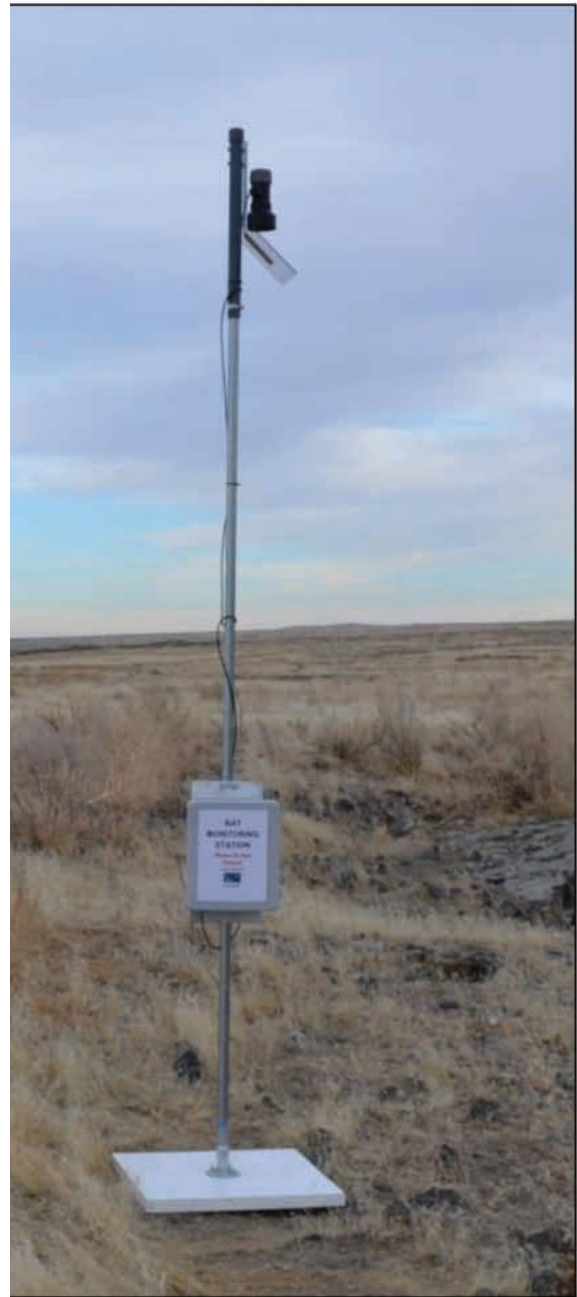
Figure 9-9. A Passive-Acoustical Monitoring Station for Bats with a Microphone Mounted at the Top (these devices record the echolocation calls of bats).
