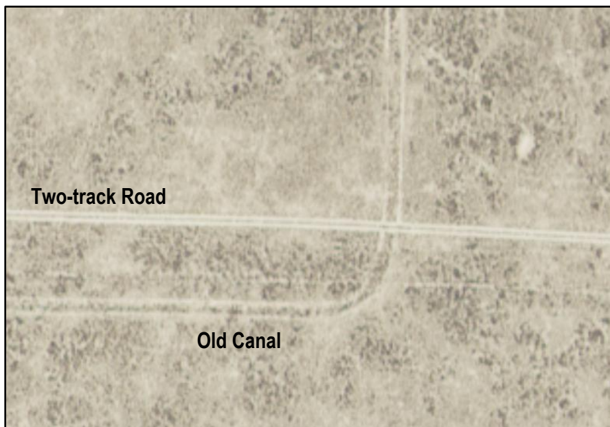
Figure 4-7. An example image subset showing two different linear disturbance features on the INL Site. The width of the features can be used to distinguish two-track roads from other features.
