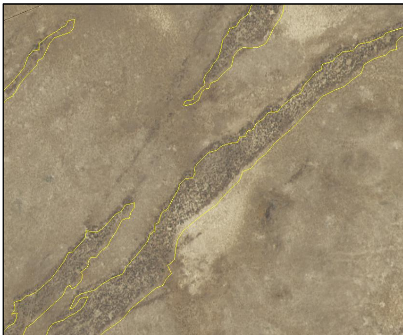
Figure 3-5. The yellow polygons were originally produced in the fall of 2010 using the 2010 GeoEye-1 basemap imagery. They are plotted here on the 2013 Idaho NAIP imagery and the slight offset to the southeast between the delineated edge and the vegetation patch edge is evident.
