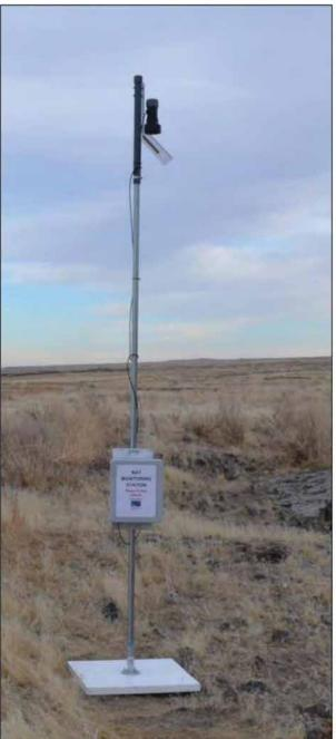
Figure 9-8. A Passive-acoustical Monitoring Station for Bats with a Microphone Mounted at the Top. These Devices Record the Echolocation Calls of Bats.
