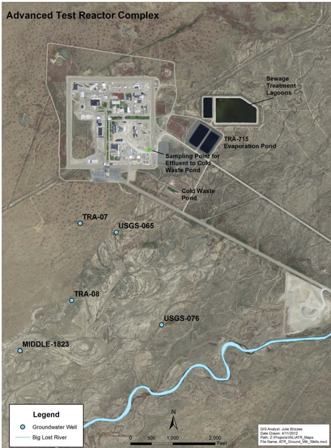
Figure 5-1. Permit Monitoring Locations for the ATR Complex Cold Waste Pond.
