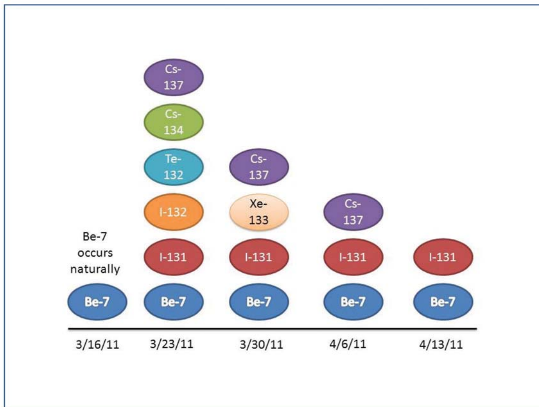
Figure B-2. Gamma-emitting Radionuclides Detected in INL Site Environmental Monitoring Program Air Filters.
