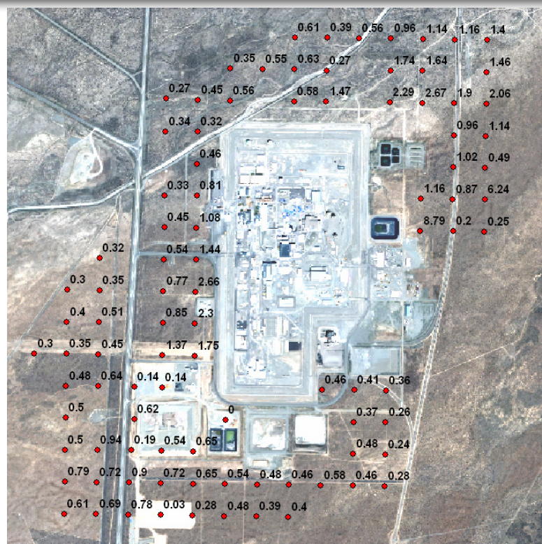
Figure E-4. 2006 In Situ Gamma Scan Results (pCi/g) for 137 Cs at INTEC.
