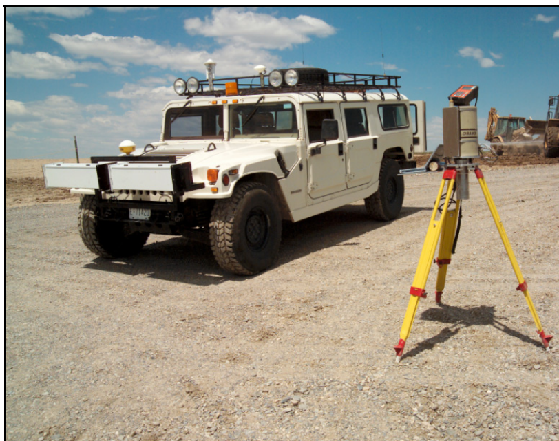
Figure E-1. Global Positioning Radiometric Scanner (GPRS) and In Situ Gamma-Ray Spectrometry System.
