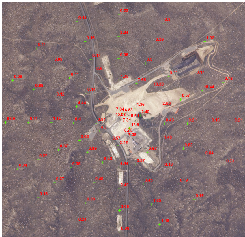
Figure E-9. 2006 In Situ Gamma Scan Results (pCi/g) for ^{137}\text{Cs} at ARA.
