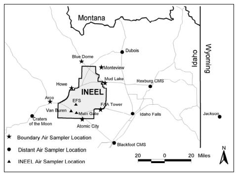
Figure 1. Low-volume air sampler locations.
