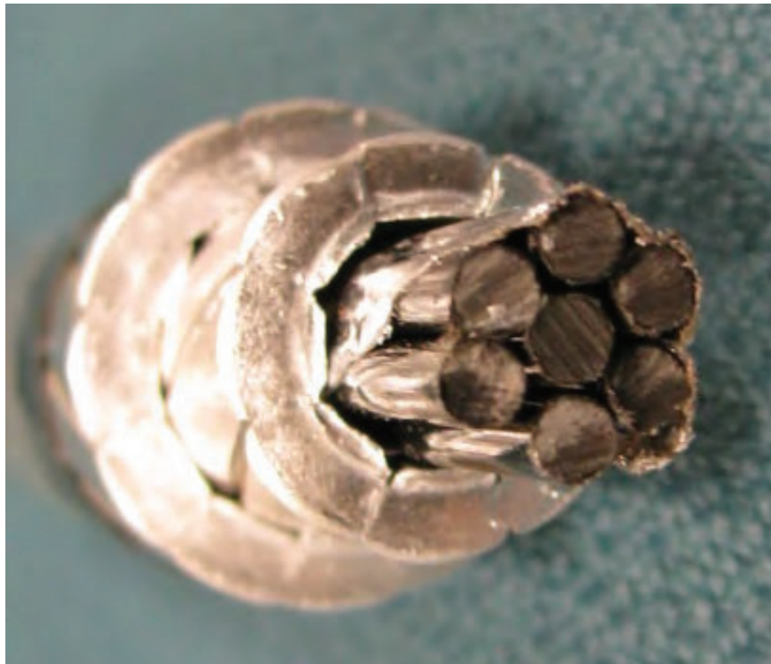
Figure 2-61. Southwire aluminum conductor carbon fiber core reinforced (ACCR), C 7 -TP cross-section
