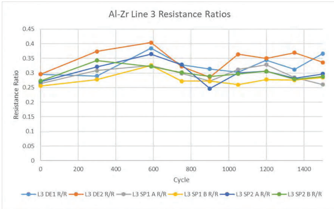
Figure 2-65. ACCR C 7 -TP Line 3 resistance ratios throughout thermal cycling process
