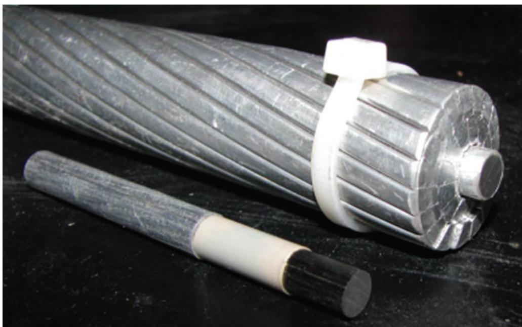
Figure 2-44. Nexans Lo-Sag conductor cross-section
