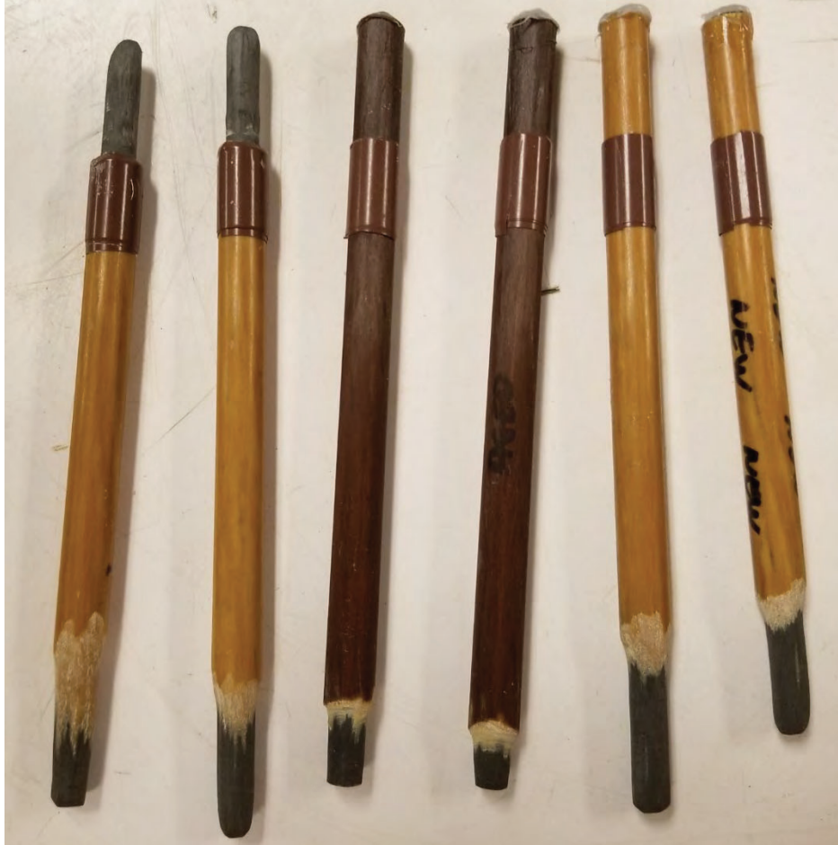
Figure 8-3. CTC cores prepared for testing: exposed core from new conductor (2 left samples), coated core from aged conductor (2 middle samples), and coated core from new conductor (2 right samples).
