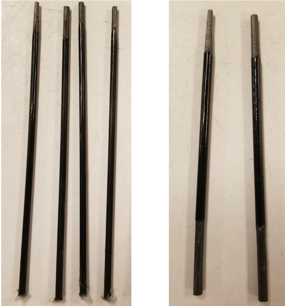
Figure 8-2. Coated Southwire C7 carbon strands (left) and uncoated Southwire C7 carbon strands (right).
