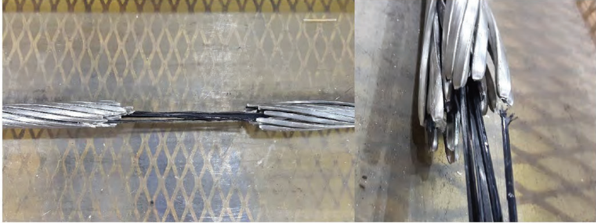
Figure 4-20. T13 ZTACCR/TW/C 7 (Southwire ACCR C 7 ) conductor at failure location for high temperature test
