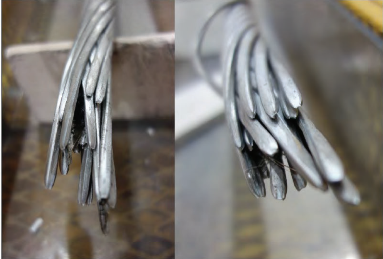
Figure 4-25. T13 ACCS/TW/C 7 (Southwire ACCS C 7 ) conductor at failure location for high temperature test
