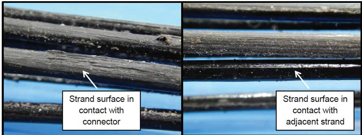
Figure 3-15. Surface Condition of Organic Composite Core Strands from Celanese ACCS C 7 -TW after Failure
